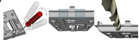
On the upper side of the base plate there are 2 grits as position for a drill hole max. Ø 6 mm
